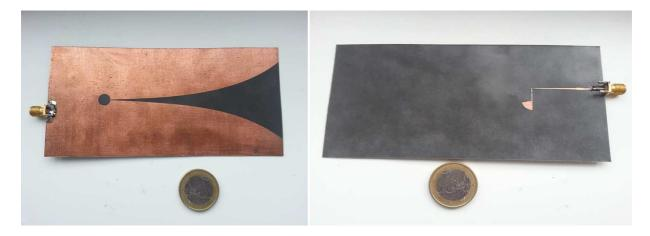
✓ Demonstration of the front and back end of the antenna to be used for the reconfigurable network demonstrator
